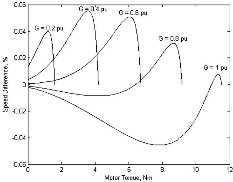
**Figure 9.** Speed difference-torque characteristics of the shunt DC motor.
