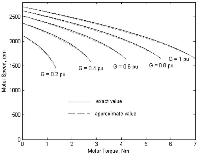
**Figure 11.** Speed-torque characteristics of the separately excited DC motor.
