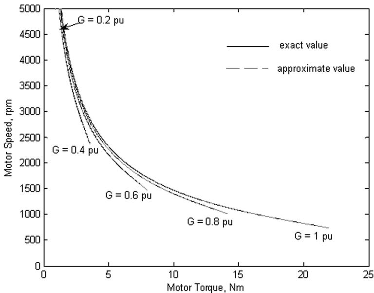
**Figure 4.** Speed-torque characteristics of the series DC motor.
