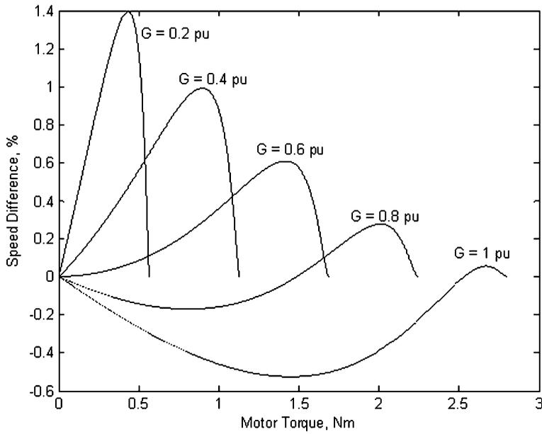
**Figure 8.** Speed difference-torque characteristics of the separately excited DC motor.
