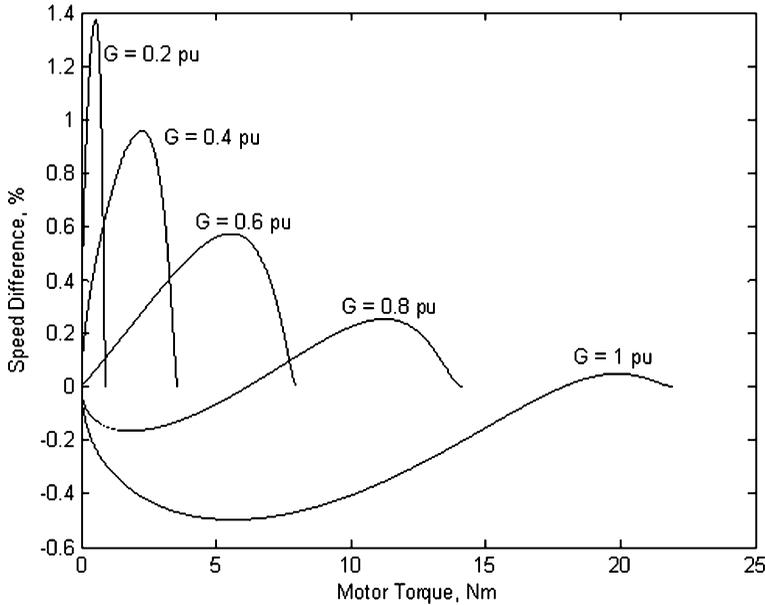
**Figure 7.** Speed difference-torque characteristics of the series DC motor.
