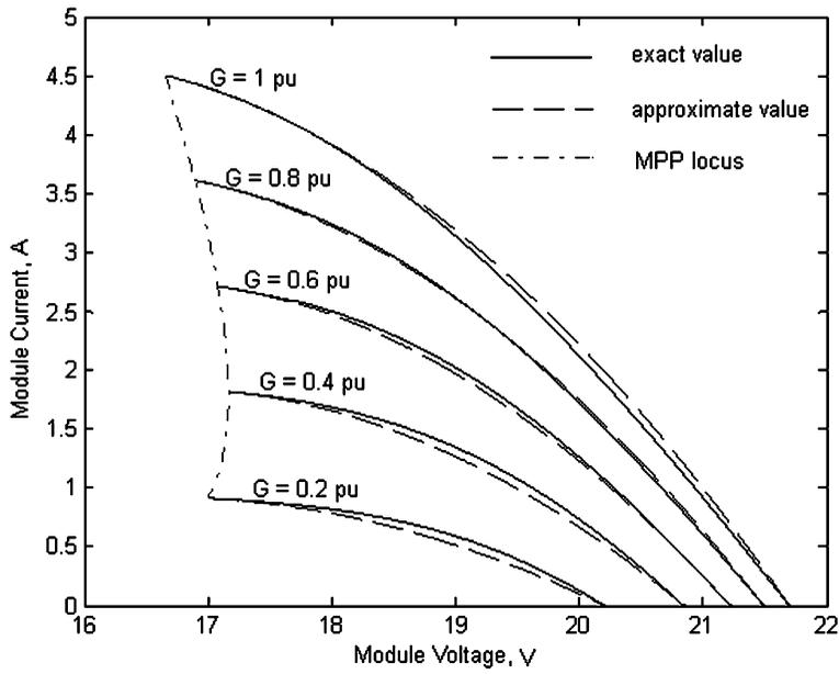
**Figure 2.** Comparison between exact and approximate current-voltage characteristics of a PV module at different insolation levels.
