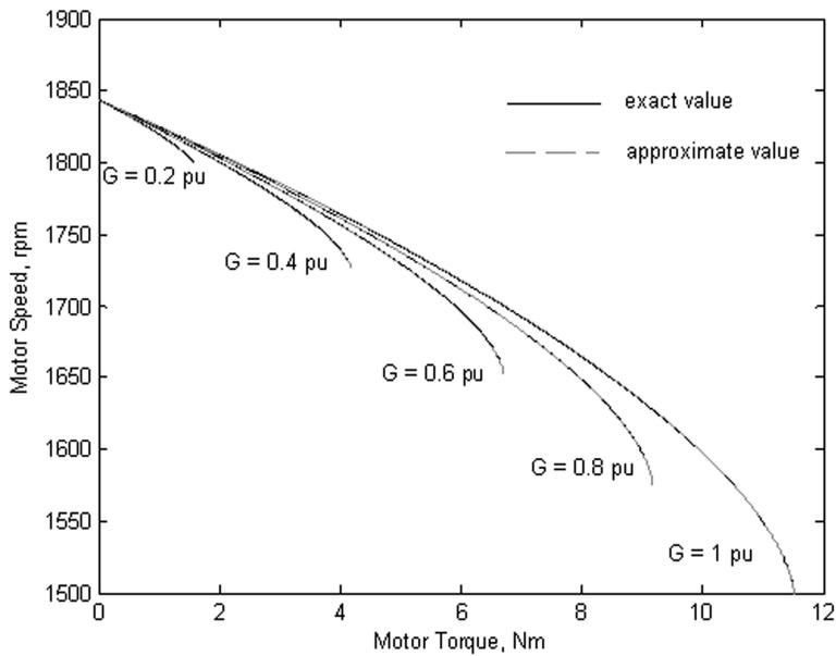
**Figure 6.** Speed-torque characteristics of the shunt DC motor.
