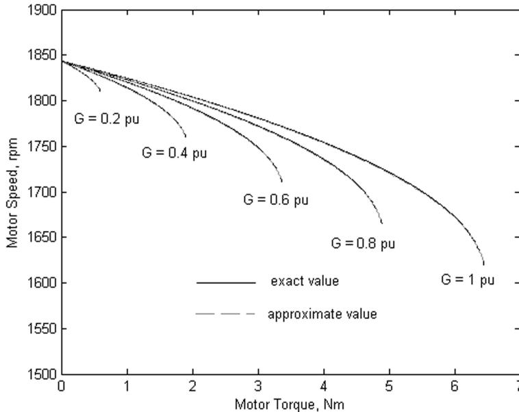
**Figure 12.** Speed-torque characteristics of the shunt DC motor.
