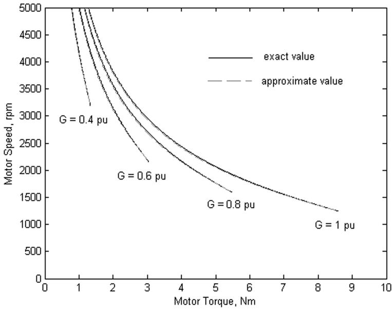
**Figure 10.** Speed-torque characteristics of the series DC motor.
