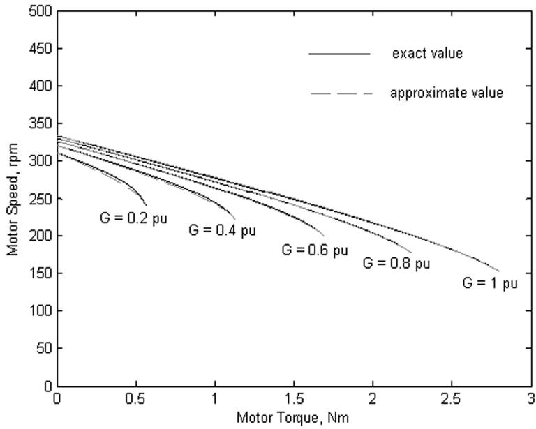
**Figure 5.** Speed-torque characteristics of the separately excited DC motor.
