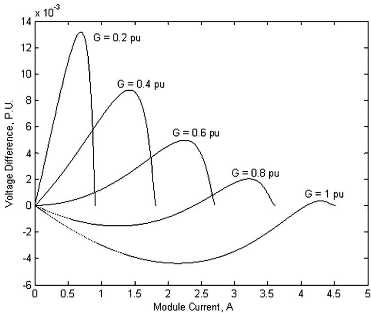
**Figure 3.** Voltage differences versus current of a PV module at different insolation levels.
