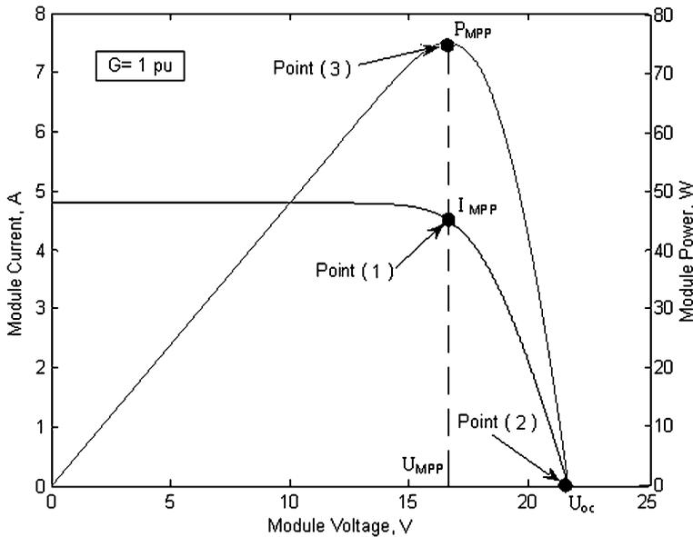
**Figure 1.** Current-voltage and power-voltage characteristics of a PV module.
